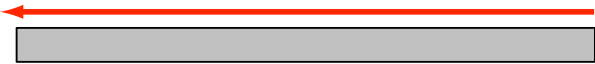
Figure 10.2: This picking area contains only popular skus and so every order is likely to require walking down the aisle. Thus an efficient route of travel is known in advance.
