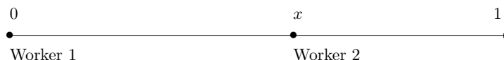
Figure 11.2: Positions of the worker 2 immediately after having completed the k -th order and walked back to take over the order of worker 1 (who has walked back to the start of the line to begin a new customer order).
