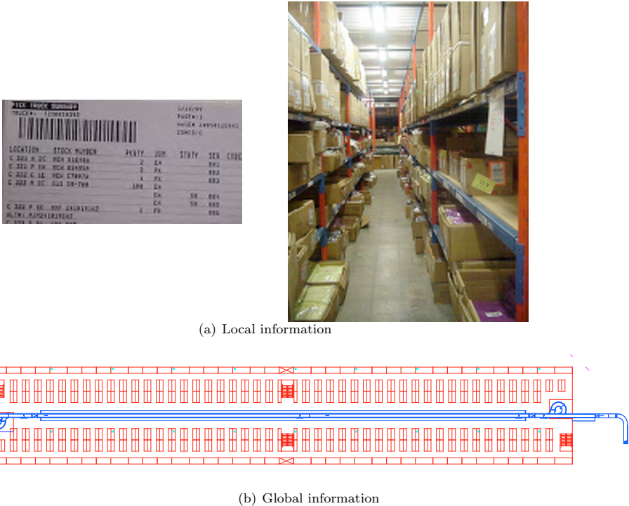
Figure 10.1: An order picker has only local information, such as a sequence of locations and the view from an aisle (a), from which to determine a pick path that is globally efficient. It is hard for the order picker to know or account for the global layout of the pick area (b).
