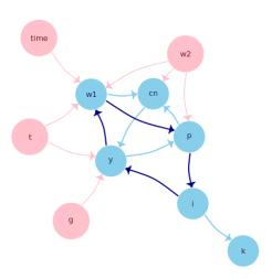
Each edge states a simultaneous dependence from a variable to another, e.g. the w1 equation depends on the current value of the time time series; complexity arises because in this model there are several circular dependencies, one of which is plotted in dark blue.
